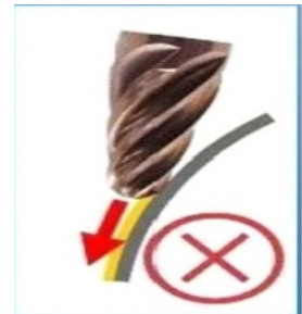
Avoid feeding downward with the tool tip.
