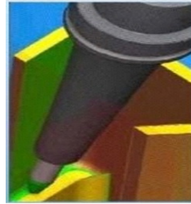
Use the tip radius for small corner-cleaning operations.
