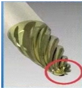
Avoid the bottom tip area when chip space is limited.
